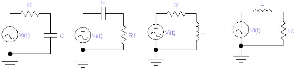
$$1) V_C(s) = V_i(s) \cdot \frac{\frac{1}{sC}}{R + \frac{1}{sC}} = V_i(s) \cdot \frac{1}{1 + sRC} = V_i(s) \cdot \frac{1/RC}{s + 1/RC} = V_i(s) \cdot \frac{\omega_t}{s + \omega_t}$$
